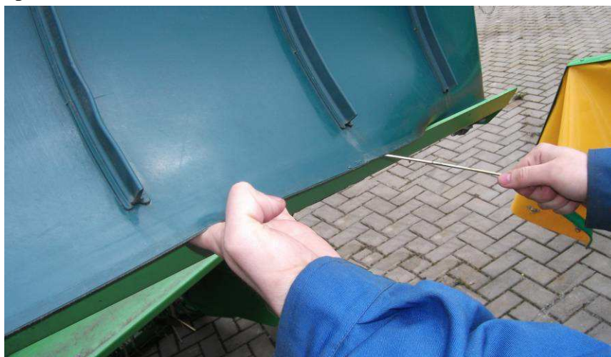
Fig. 28. Removal of impurities inside the conveyor belt
